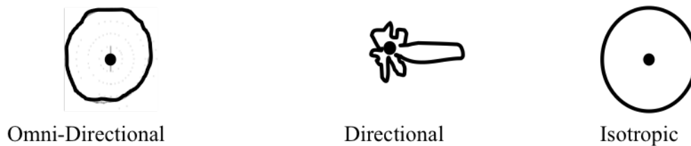
Figure 3.1 Different types of antennas
